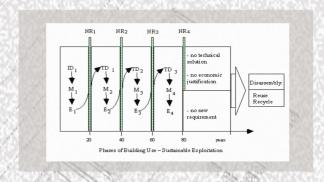
Sustainable design should be focused on juxtaposition of the materials and functions of building parts at joints. The interface between components plays a crucial role in re-assembly, which is an ultimate form of recycling and reusing. In that respect the development towards systematisation and modulation of building parts into subsystems presents the way to achieve more effective buildings with controlled use of energy, raw materials and less man-power [Horden98].
